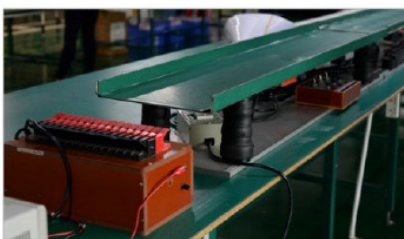
Vibration test table Vibrate the finished products , for testing the stability of the products
