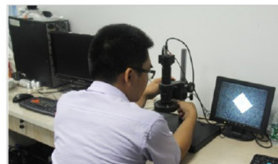
Microscope Observe the LED sources are intact
