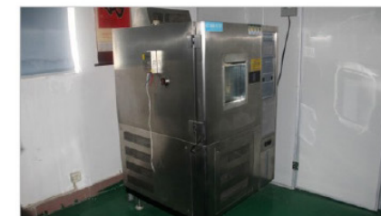
Constant temperature and humidity chamber (-20°C ~ 50°C) Test fixtures performance in harsh environment
