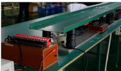
Vibration test table Vibrate the finished products, for testing the stability of the products
