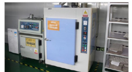
LED electric oven Remove the moisture from the LED sources, to keep the good stability of the LEDs, otherwise, with the moisture inside the LED, the LED easy to broke during usage
