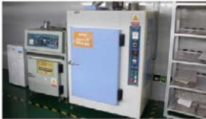
LED electric oven Remove the moisture from the LED sources, to keep the good stability of the LEDs, otherwise, with the moisture inside the LED, the LED easy to broke during usage
