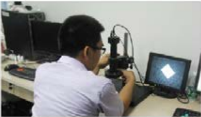
Microscope Observe the LED sources are intact
